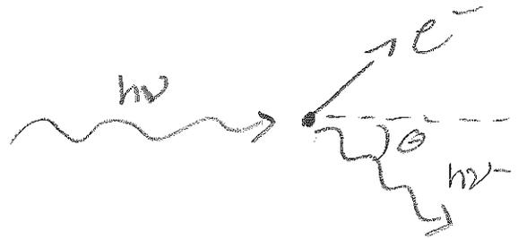
where  $\lambda_c = \frac{h}{m_e c} = \text{Compton wavelength} = 2.4 \times 10^{-10} \text{ cm}$  Short wavelength
